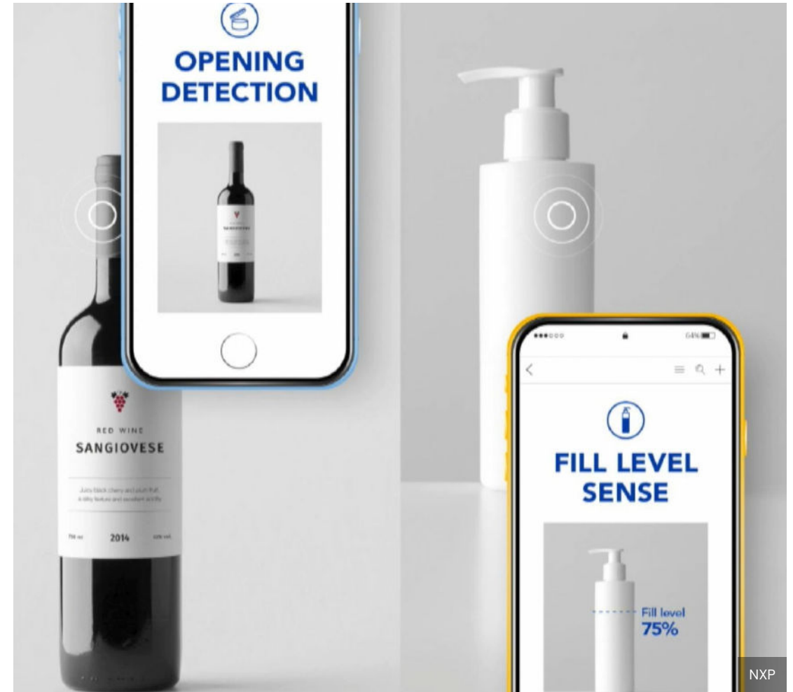
NXP (Netherlands) showcased the possibilities of its NFC chip-based system, which allows brands and consumers to detect whether a product has been opened already plus the current fill level
