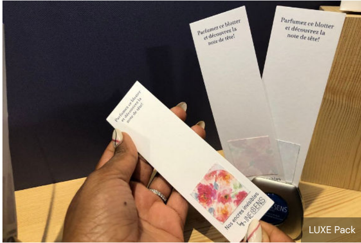
French label specialist InessenS has created a paper for fragrance testers which reacts to perfume, revealing a pattern, to avoid accidental reuse of tester sticks
